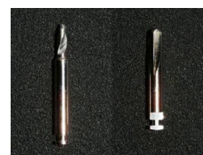
FIGURE 2. Adapted drill of 1.6 × 5.0 mm and adapter for key pad.
